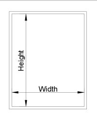
Measure inside of the window trim, always measure width first then height and write it down in that order, also please use inches. If the window is longer then 108" the blind will need to be split in two at the mullion, (see illustration)
